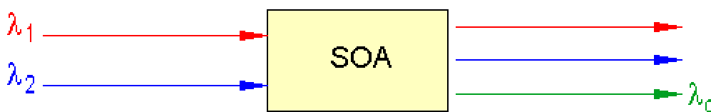
Figure 7: Schematic of the Four Wave Mixing (FWM) process.
